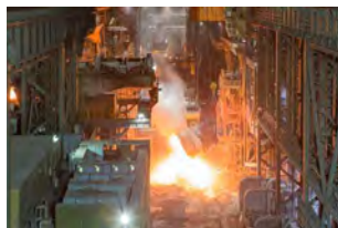
High pressure phosphorus removal in steel works
