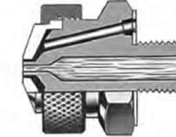
External mix with pressure set-ups: round spray patterns
