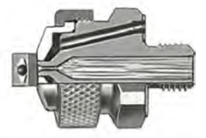
External mix with pressure set-ups: flat spray patterns
